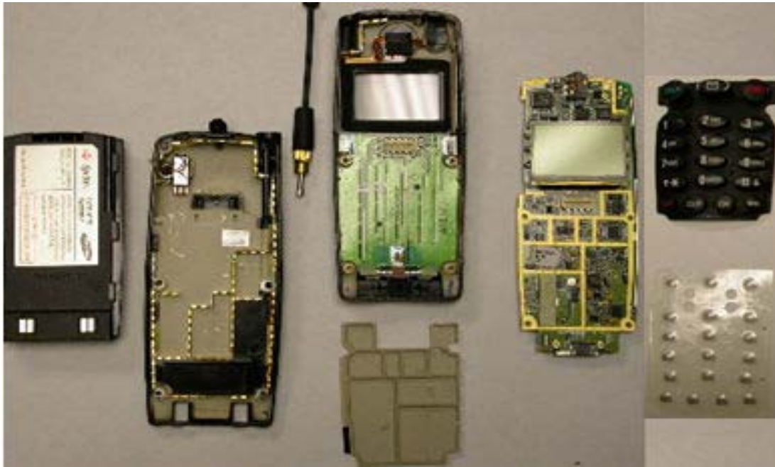
Fig.1 Typical components of a mobile phone. [26]
